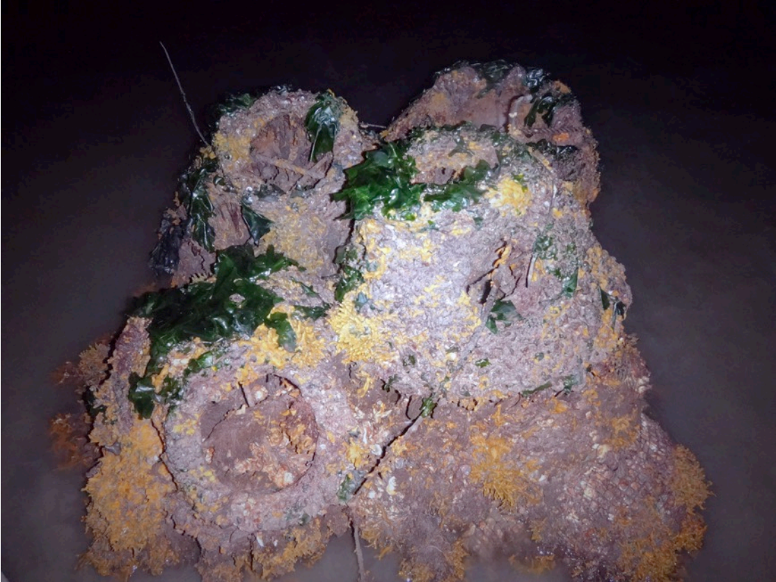
Figure 26. Small reef ball stack at TNC site is collapsing.
